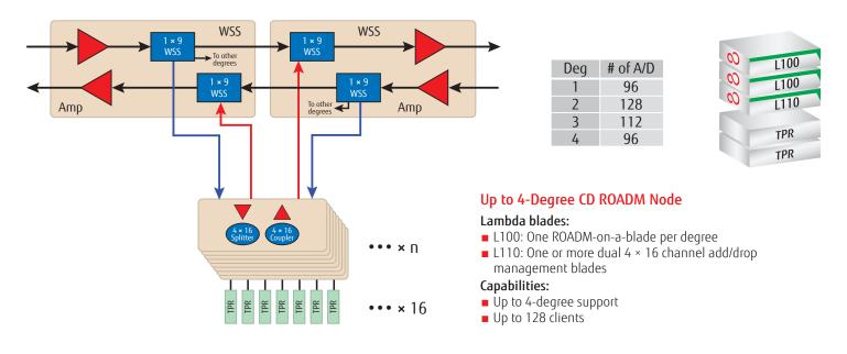
Up to 4-degree CD-ROADM node configuration with transponders (TPR)
